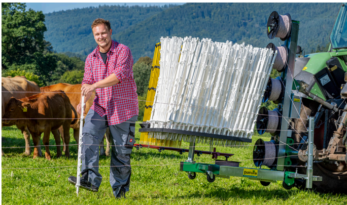
Exchangeable magazine for up to 400 posts
